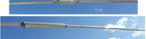
Make sure to have heach one tubes connection having bolts head on the same side.
